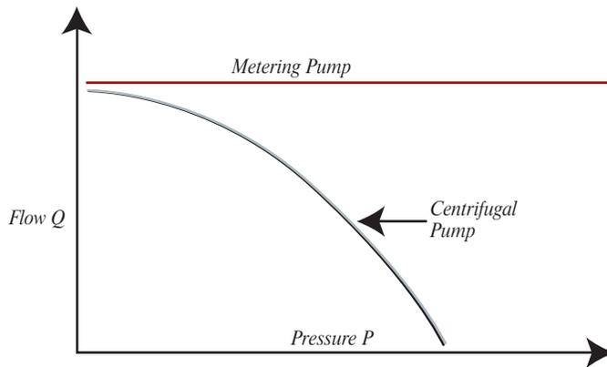
2. Unlike centrifugal pumps, flow rate is not greatly affected by changes in discharge pressure.
